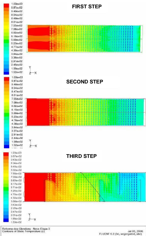
**Figure 5. EVOLUTION OF THE TEMPERATURE PROFILE OF THE COMBUSTION GASES – UPPER VIEW**
