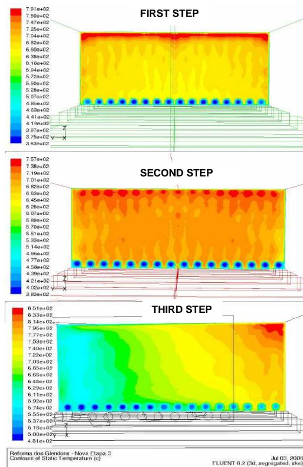
**Figure 6. EVOLUTION OF THE TEMPERATURE PROFILE OF THE COMBUSTION GASES – CROSS SECTION VIEW**
