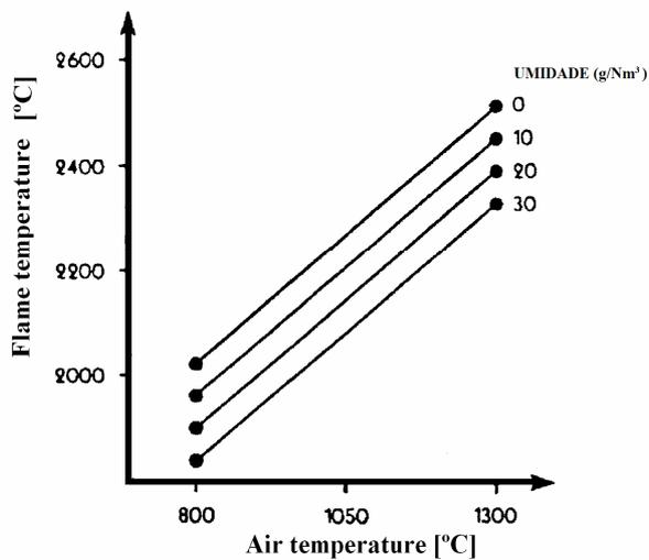
**Figure 2. EFFECT OF AIR TEMPERATURE ON THE COMBUSTION FLAME TEMPERATURE**
