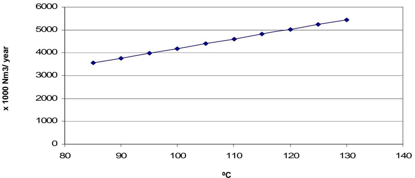
Figure 7 ANNUAL SAVING OF OXYGEN AS A FUNCTION OF AIR TEMPERATURE INCREASE
