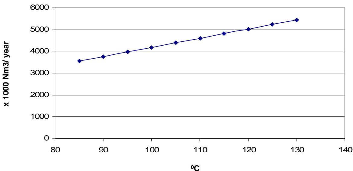
Figure 6. Annual saving of oxygen as a function of air temperature increase
