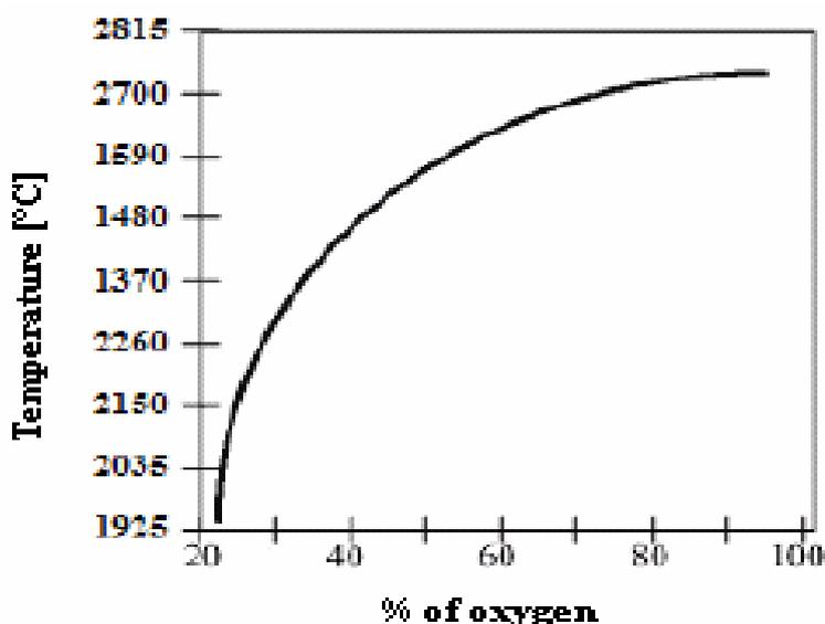
Figure 1. Effect of the oxygen concentration on the combustion flame temperature
